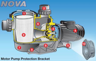
Situated between the pump wet end & the pump motor, a mechanical seal forms a seal around the motor shaft to prevent water from travelling along the motor's shaft.
